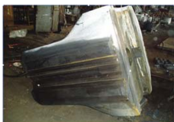
10T模锻锤锤头断裂修复
